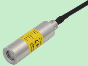
SS636 series features a big open 316L stainless steel corrugated diaphragm, is easy for daily maintenance. The sensors give a long term and accurate readings at pressure ranges from 100 mBar up to 5 Bar in the measurement of level and depth (corresponding to water column depths of 1 m to 50 m). Typical applications including river level, tank level, borehole level, aquifer level and environmental monitoring.
