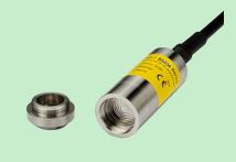
The electrical connection is a special designed PU or PE cable with air tube and the pressure connection part is an exposed 316L stainless steel corrugated diaphragm, no pressure port and no blocking problems, easy for daily maintenance. Typical applications including water and sewage treatment plants, water level monitoring at reservoirs, dams, down-hole water wells.
