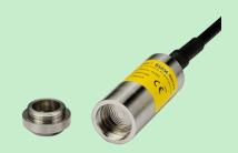
The electrical connection is a special designed PU or PE cable with air tube and the pressure connection part is an exposed 316L stainless steel corrugated diaphragm, no pressure port and no blocking problems, easy for daily maintenance. Typical applications including water and sewage treatment plants, water level monitoring at reservoirs, dams, down-hole water wells.
