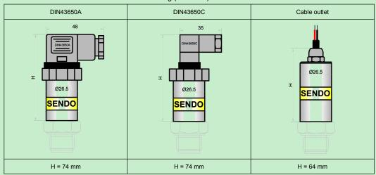
Dimensions for electrical connections and housing (Unit: mm)
