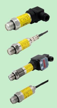
spanning from 0.1 bar up to 1000 bar with amplified voltage or current outputs. SS402 series is highly configurable, with a variety of electrical termination and flush pressure port configurations, the sensor is ideal used in food process and industrial applications to measure the liquid and gas pressures, where the media is either viscous, or is otherwise liable to block the port of a conventional pressure transducer with a recessed diaphragm or pressure port.
