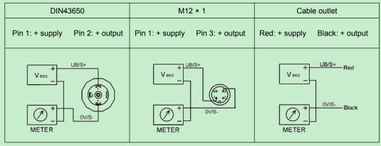
Electrical connections for 0-10V, 0-5V, 0.5-4.5V voltage output signal (3 wire)
